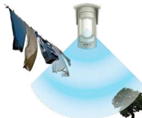
With active SCP function: the signals of the two PIR are not homogenous; no alarm is triggered off
